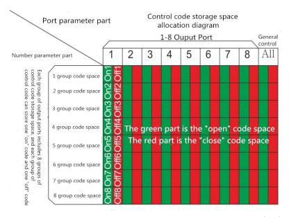
The feature of supporting simultaneous control of multiple control codes provides more flexibility and practicability for applications
